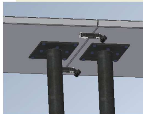
Latch in connected position
